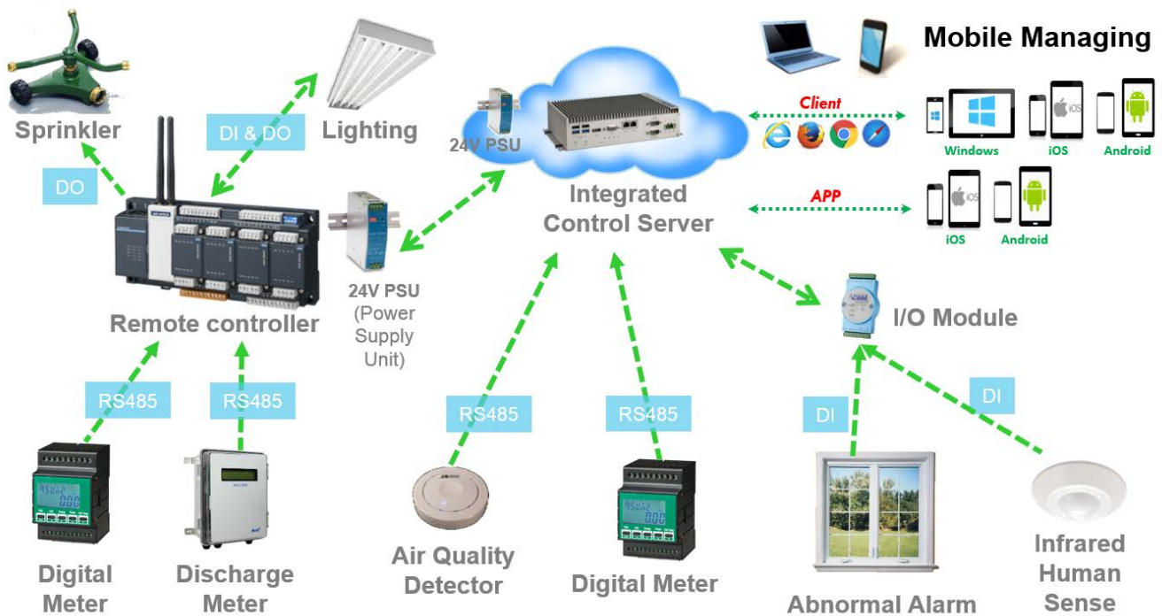
Figure 2. Simple building central control technology architecture
